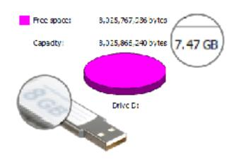
This is because storage is advertised as a power of ten (10<sup>9</sup> for giga-) but the digital devices work using binary (0s and 1s - only two **bi**nary digi**ts** - or bits, with 8 bits in a byte)\*. Finish the table:
